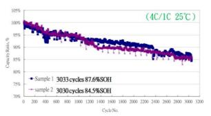
The typical cycle life was tested in lab under controlled environment. The field life will be fluctuated by application environment.
